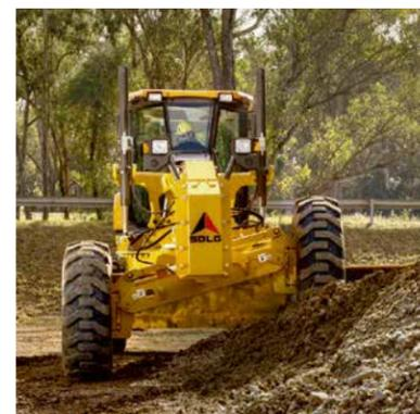
■ The frames of SDLG graders are of a box-type design to provide the best strength and durability. SDLG frames are prepared to take all attachments from the factory, for best performance. The excellent frame articulation gives you outstanding maneuverability and short turning circles.
